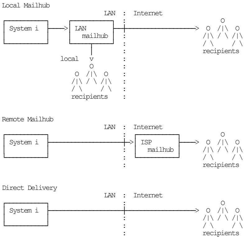
For most customers the System i is attached to a local area network that also has a mail server attached to it. Typically, the mail server runs on a PC with Exchange, Domino, SendMail, or similar mail application installed. In addition, typically, this mail server should be responsible for delivering mail, and will serve as the forwarding mailhub server for the System i. If this is your situation, proceed to the Quick Start Mail Set Up - Mailhub section.
